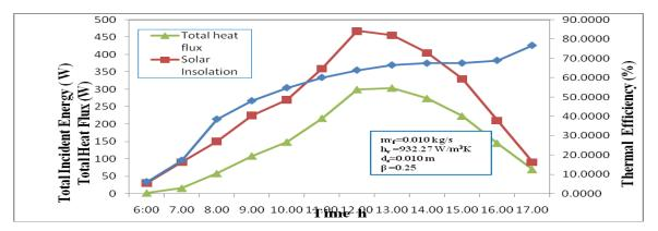
Fig: 11. Variations of Total Incident Energy, Total Heat Flux and Thermal Efficiency for Porous Marble wall with Time of the day at x=0.24 m
