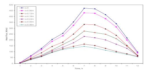
Fig: 18. Variation of Heat Flux with Wall Thickness across Brick Wall
