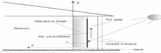
Fig: 1. Schematic diagram of 'Trombe Wall' System [1]
