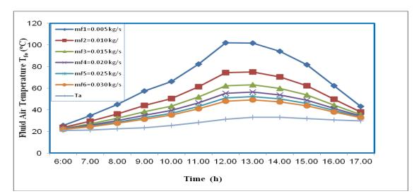
Fig: 6. Variation of Fluid (Air) Temperature for different Mass Flow Rates of air and Ambient Temperature with Time of the day
