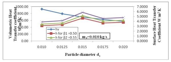
Fig: 10. Variations of Volumetric Heat Transfer Coefficient and Surface Heat Transfer Coefficient with Particle Diameter for different Porosities and a given Mass Flow Rate of air for Porous Quartzite walls
