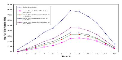
**Fig: 23.** Variation of Heat Fluxes in Brick, Concrete, Marble and Quartzite Walls at x=0.36 m and Solar Insolation with Time of the day
