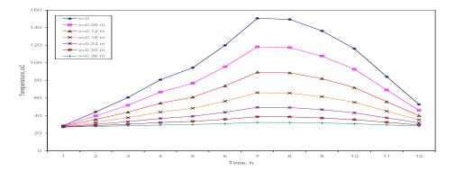
Fig: 15. Variation of Temperature across Wall Thickness for Concrete Wall
