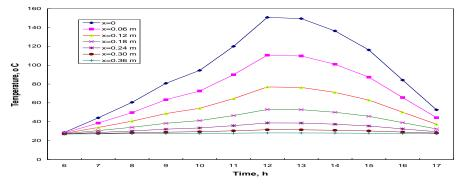
Fig: 14. Variation of Temperature across Wall Thickness for Brick Wall
