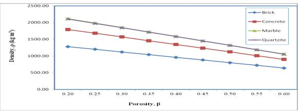
Fig: 4. Variation of Density with Porosity for different materials
