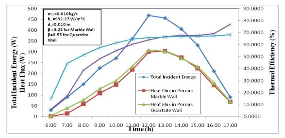
**Fig: 13.** Comparison between the variations of Total Incident Energy, Heat Fluxes and Thermal Efficiencies of Marble and Quartzite walls with Time of the day at x=0.24 m
