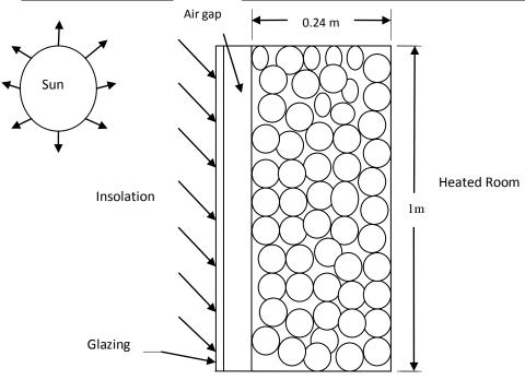
Fig: 2. Schematic diagram of a porous wall
