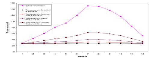
**Fig: 22.** Variation of Sol-air Temperature and Temperatures in Brick, Concrete, Marble and Quartzite Walls at x=0.36 m with Time of the day
