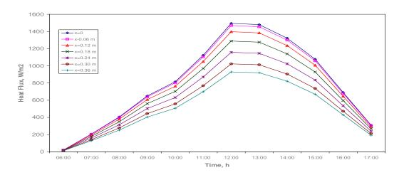
Fig: 21. Variation of Heat Flux with Wall Thickness across Quartzite Wall
