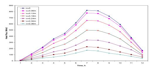
Fig. 19 Variation of Heat Flux with Wall Thickness across Concrete Wall
