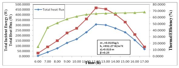
**Fig: 12.** Variations of Total Incident Energy, Total Heat Flux and Thermal Efficiency for Porous Quartzite wall with Time of the day at x=0.24 m
