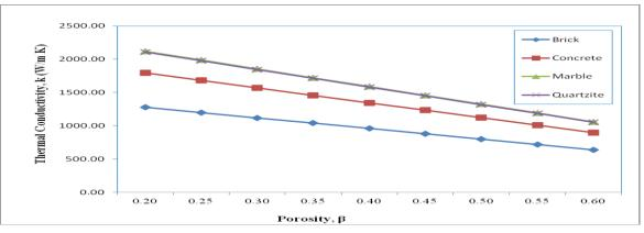
Fig: 5. Variation of Thermal Conductivity with Porosity for different materials
